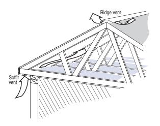
The vented area should be divided equally between the ridge and soffits.
