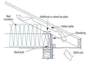
A raised top plate increases the area for insulation and ventilation at the eaves.
