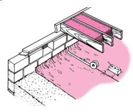
Insulate between the floor joists with R-19 batt insulation, making sure the air barrier is touching the underside of the floor, and that the insulation extends snugly against the band joist. In regard to paper-faced batts, the pink side should face toward the ground.
